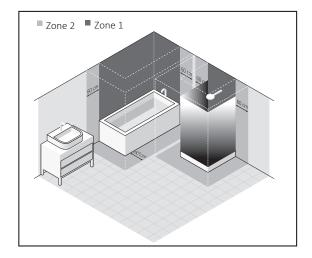
The MOA heating element can be installed in bathrooms in zone 1, 2 and outside the zones as defined by applicable law, subject to any additional regulations concerning electrical installations in wet areas.
